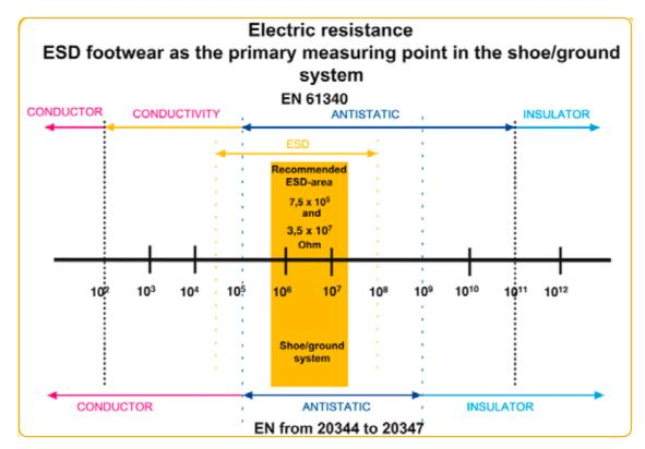
ESD shoes should be worn when there is a need to reduce the discharge load from an electrostatic charge.
